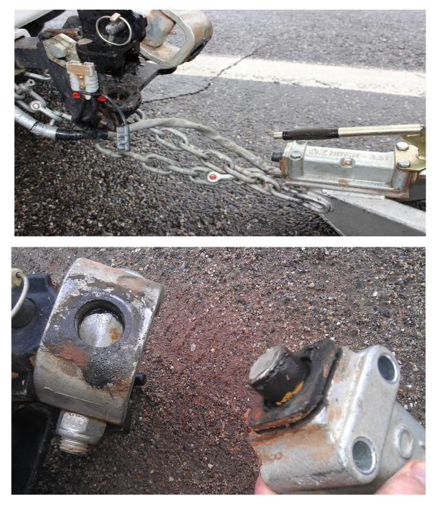
On the day of the failure, I contacted the manufacturer, Ozhitch and advised them of the situation to which they replied "we have had a few failures of these, we are happy to replace the unit". "The new units have the shaft threaded and then welded".
